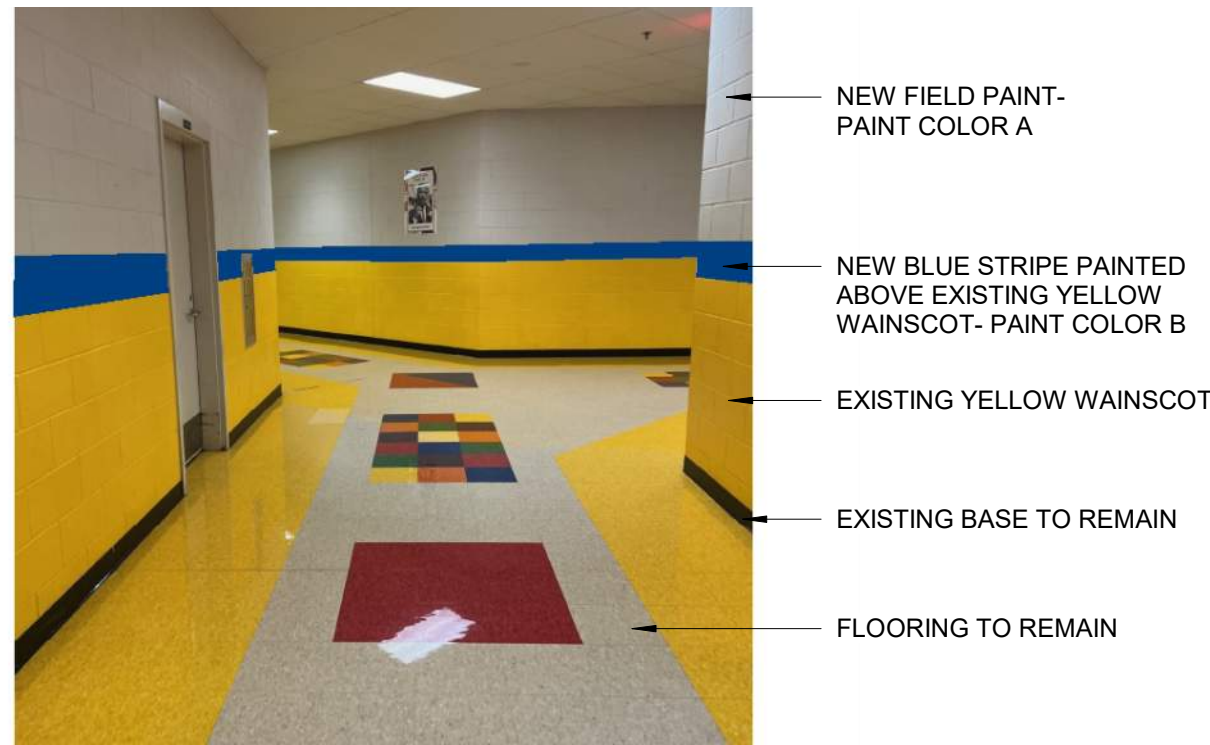
TYPICAL COMMON CORRIDOR WAINSCOT
